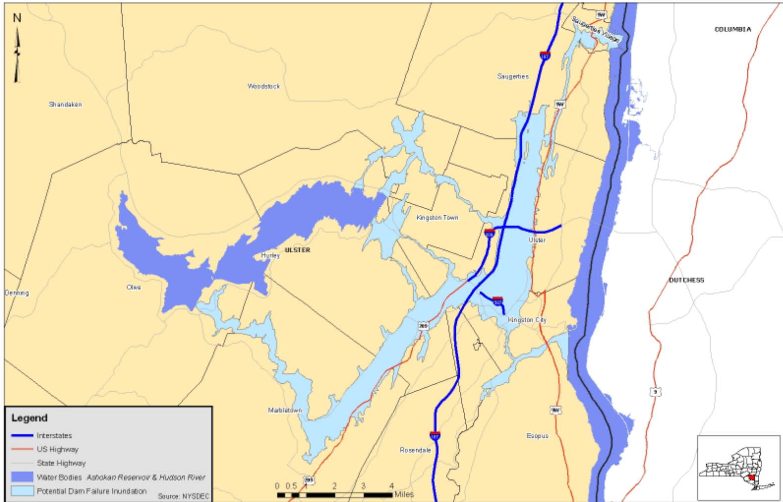
Figure 3a.9 Potential Area Affected by Failure of the Ashokan Reservoir Dam
