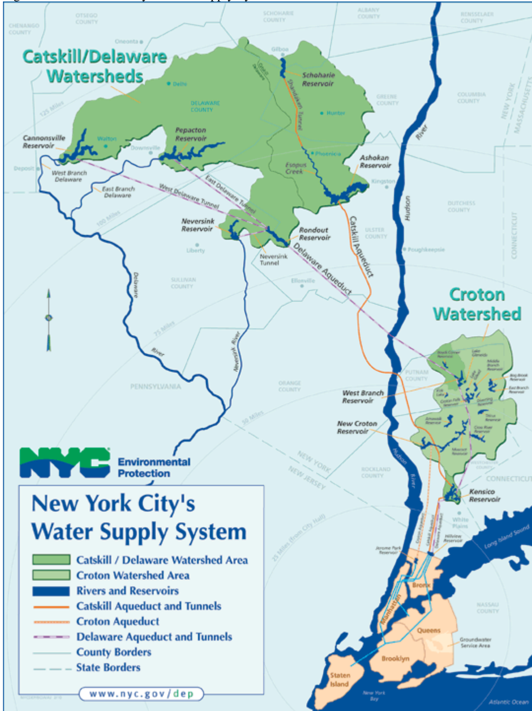
Figure 4-5. New York City’s Water Supply System
