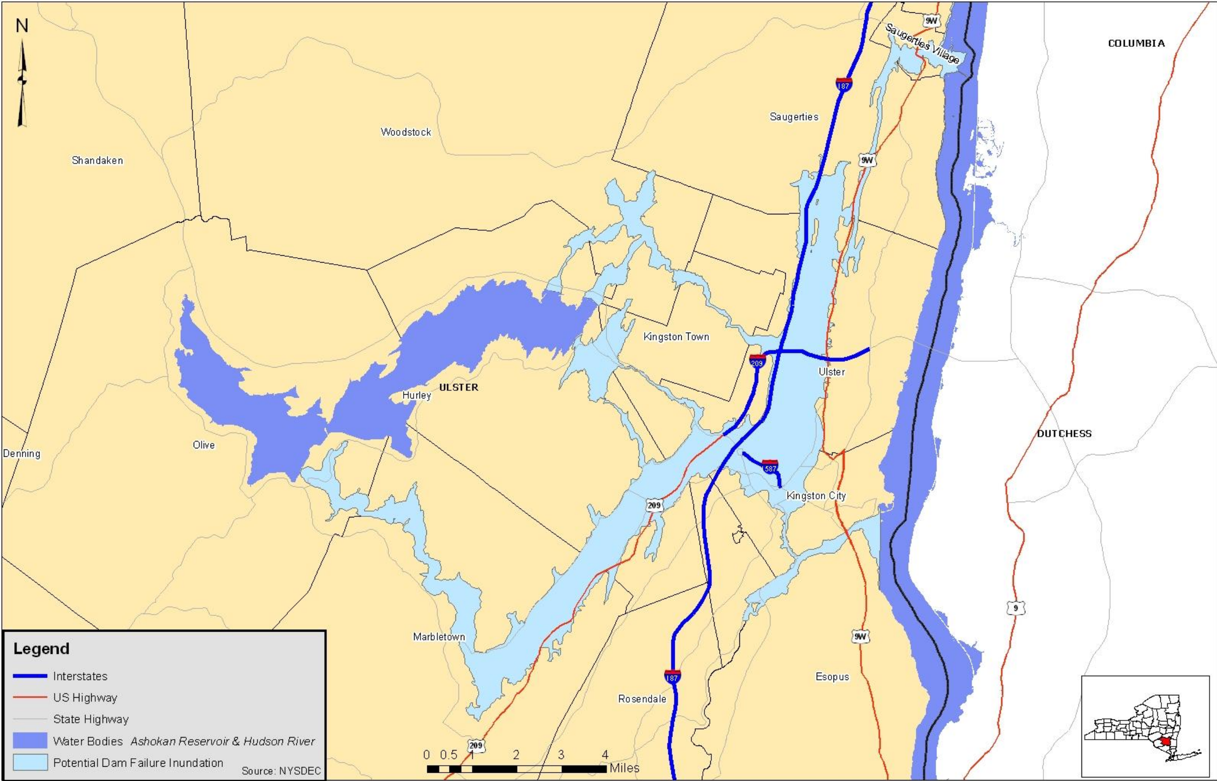
Figure 3a.6: Potential Area Affected by Failure of the Ashokan Reservoir Dam
