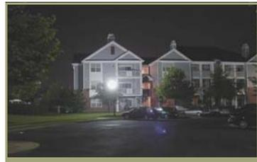
Elimination of glare is a paramount concern in most lighting designs. Luminaire viewing angles, mounting height, and shielding should all be carefully scrutinized to reduce glare. The use of unshielded wall pack units and floodlights to light parking areas or walkways should be avoided.
