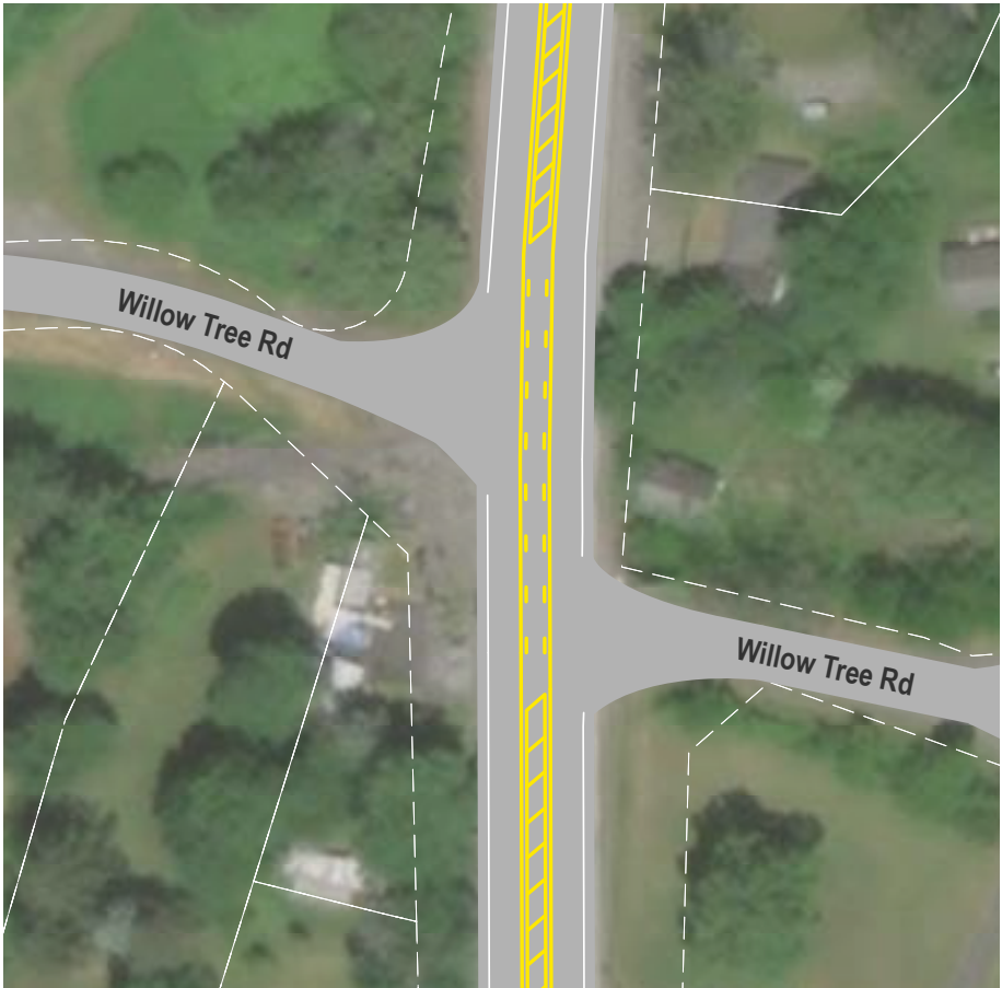
Center Turn Lane at Intersection of Route 9W and Willow Tree Road Source: BFJ Planning
