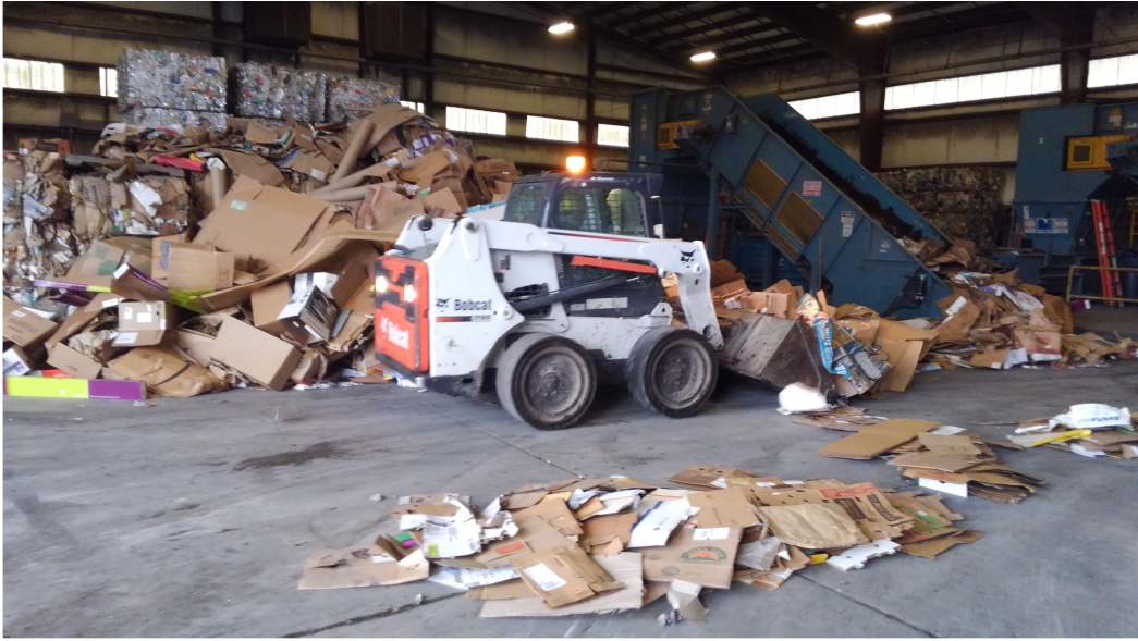
Cardboard being pushed onto a belt leading to the baler
