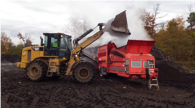
Mixture being screened
