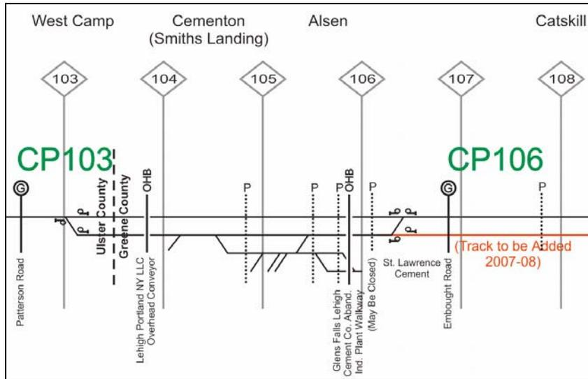
**Figure 2-22. Passing siding schematic from CP103 to CP106 at Cementon.**
