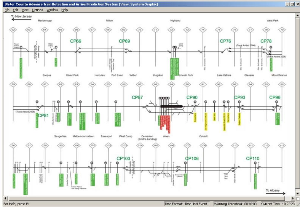
**Figure 9-5. Typical Software Screen Showing Graphical System Overview with Color-Coded Grade Crossing Predictive Status**
