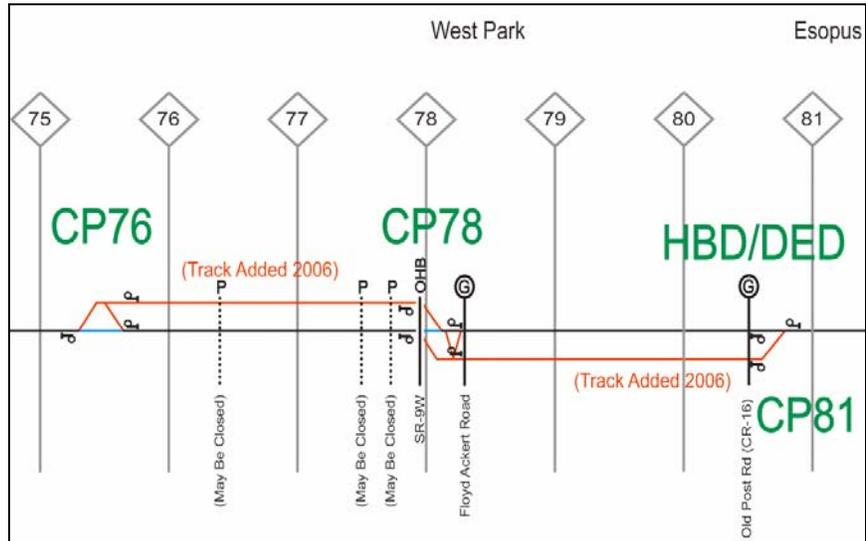
**Figure 2-17. Passing siding schematic from CP76 to CP81 at West Park.**
