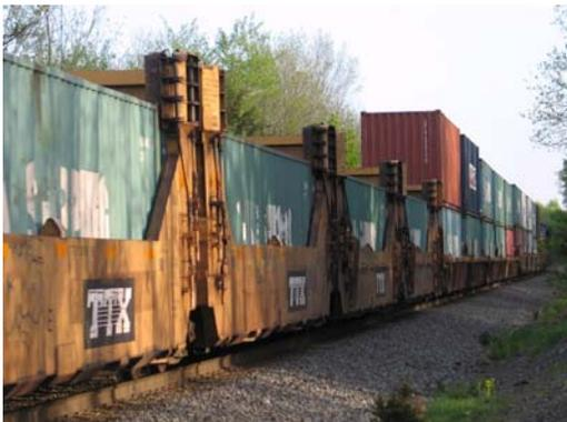
**Figure 2-10. Although multiple freight train types operate on the Corridor, the most common type is the intermodal train. This “double stack” container train is passing Patterson Road in Saugerties on its way from California to Kearny, NJ.**
