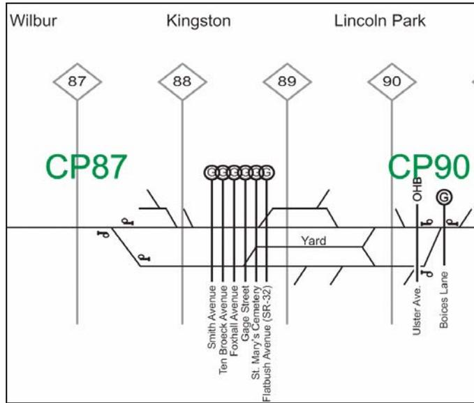
**Figure 2-18. Passing siding schematic from CP87 to CP90 at Kingston.**
