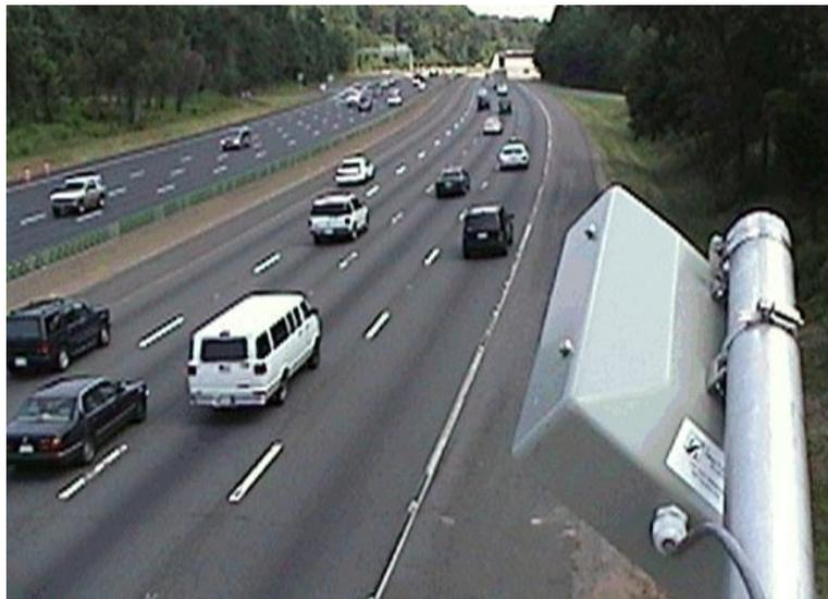
**Figure 6-2: SmarTek Systems SAS-1 Acoustic Sensor showing proximity to highway traffic.**
