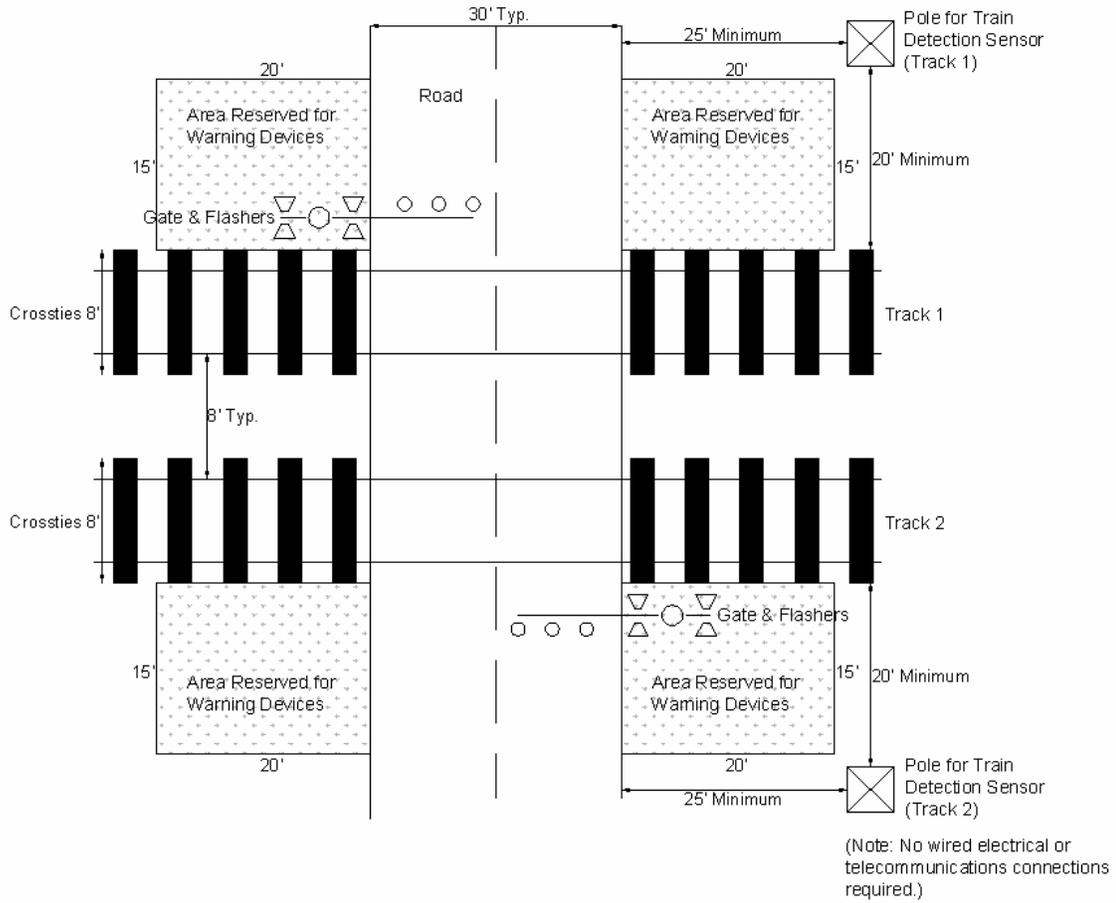
**Figure 6-7: Potential Installation Configuration for Doppler Technology in Double-Track Territory.**
