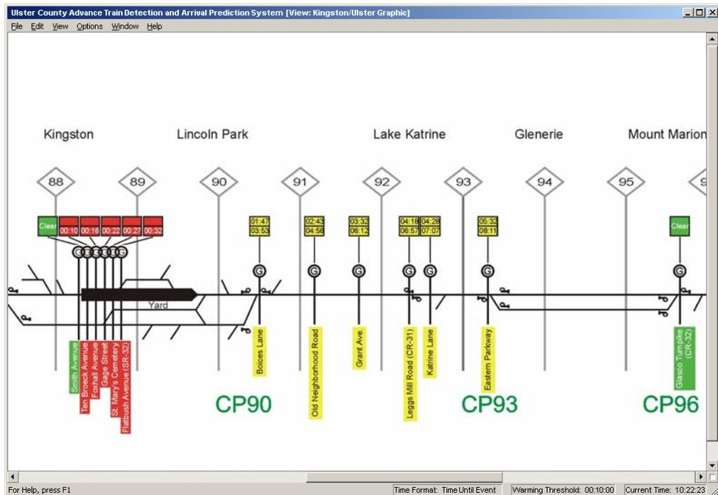
**Figure 9-6. Typical Software Screen Showing Graphical System Zoom with Color-Coded Grade Crossing Predictive Status and "Time to Go" Predictive Information in Text Boxes**
