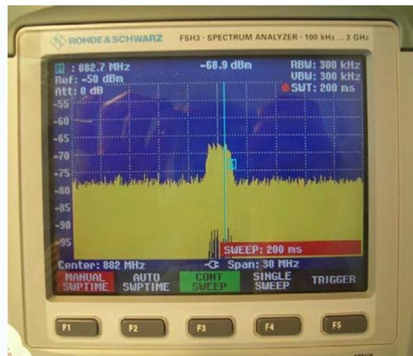
**Figure 3-5. Typical cell phone signal strength reading, showing -68.9 dBm value.**
