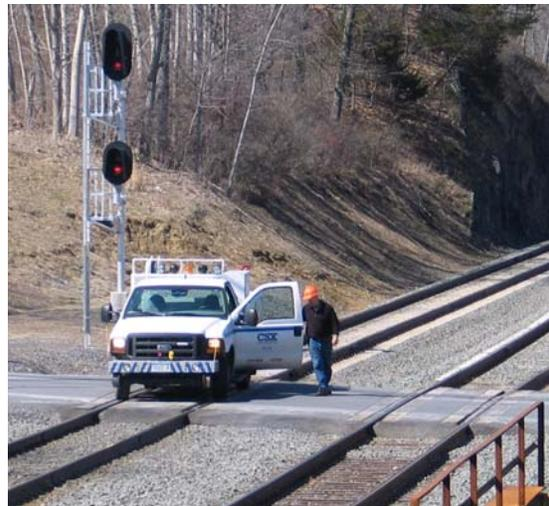
**Figure 2-9. In addition to train movements, the CSX River Line includes numerous “hi-rail” (highway vehicles with deployable rail wheels) vehicles for inspection and maintenance activities. This hi-rail vehicle is operating on the railroad at Old Post Road in Esopus.**
