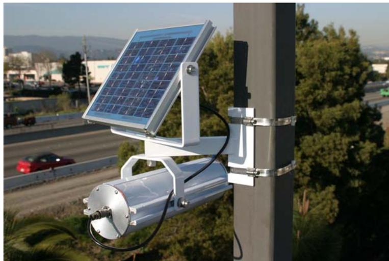
**Figure 6-4: SpeedInfo Doppler Radar Speed Sensor DVSS-100 and supporting solar panel**
