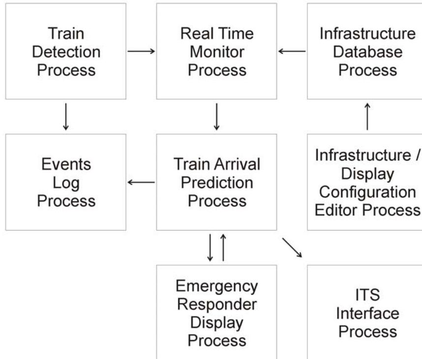
**Figure 9-2. Recommended System Software Architecture**
