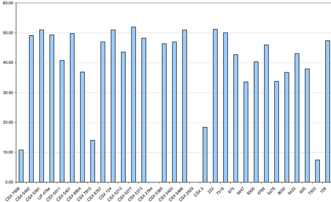
**Figure 2-20. Train speeds between Wiltwyck Cemetery and Boices Lane, calculated from September 19-20, 2007 field observations.**
