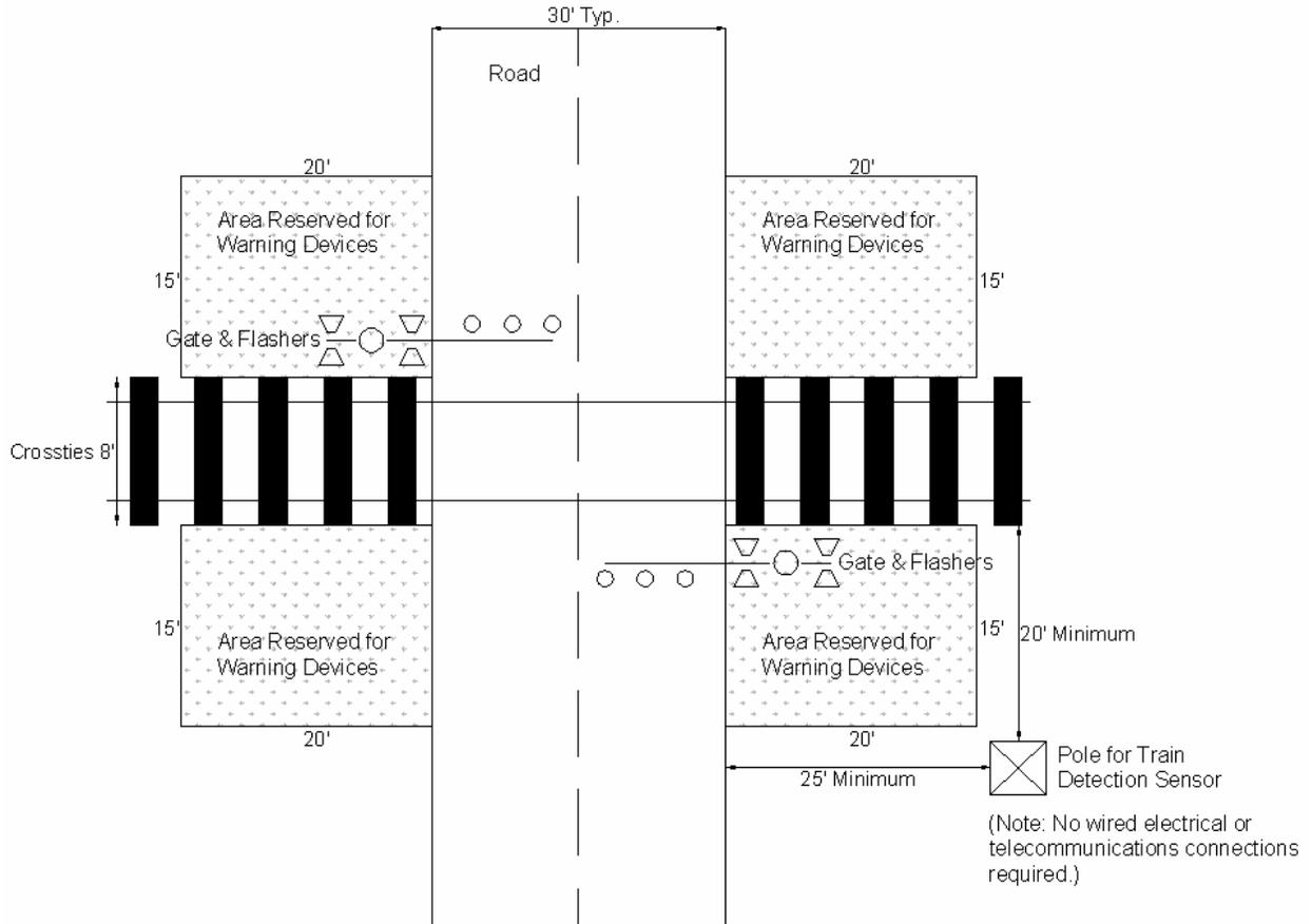
**Figure 6-6: Potential Installation Configuration for Doppler Technology in Single-Track Territory.**
