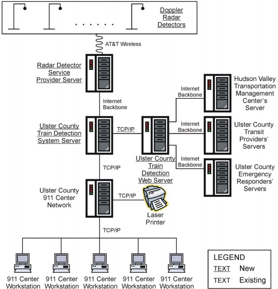
**Figure 9-1. Recommended System Hardware Architecture**
