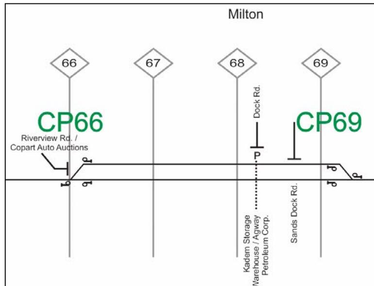
**Figure 2-15. Passing siding schematic from CP66 to CP 69 at Milton.**
