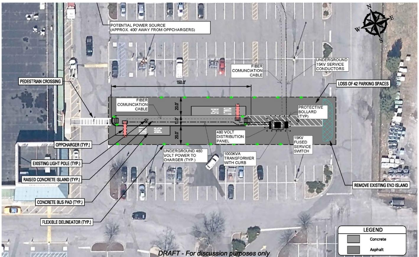
It is assumed that the existing bus stop would be relocated to and consolidated with the proposed charging station island. Different than the other two alternatives this option includes a single 150 feet long raised curb island with 2 pantograph chargers on each end. An 11-foot wide center island could be
