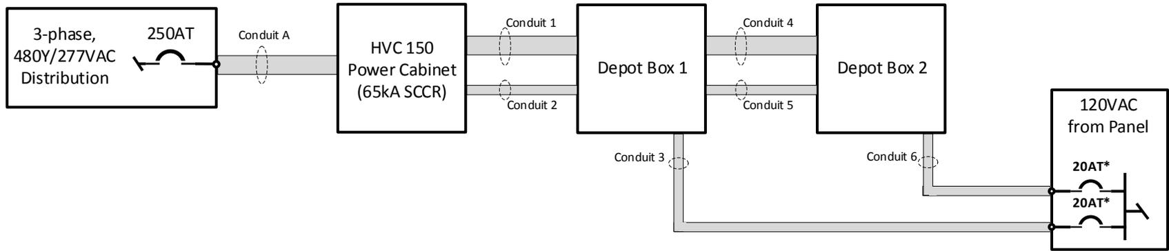
\* Control power feeds to depot boxes must have 30mA Ground Fault Circuit Interrupter and support max inrush current of 100A for < 5ms
