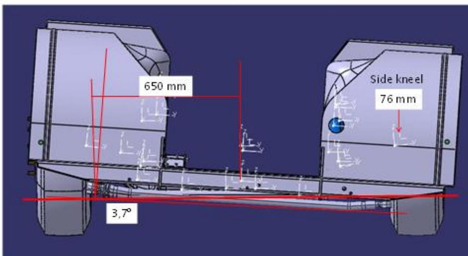
Low rotation in z-dir – estimated on the ground and 650 mm to the side in y-dir.
