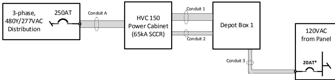
\* Control power feeds to depot boxes must have 30mA Ground Fault Circuit Interrupter and support max inrush current of 100A for < 5ms
