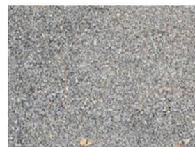
**COMPACTED CRUSHED STONE**
