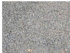
**COMPACTED CRUSHED STONE**
