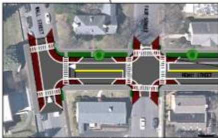
RED TEXTURED CURB EXTENSION DETAIL WALL STREET AND PARK STREET INTERSECTION
