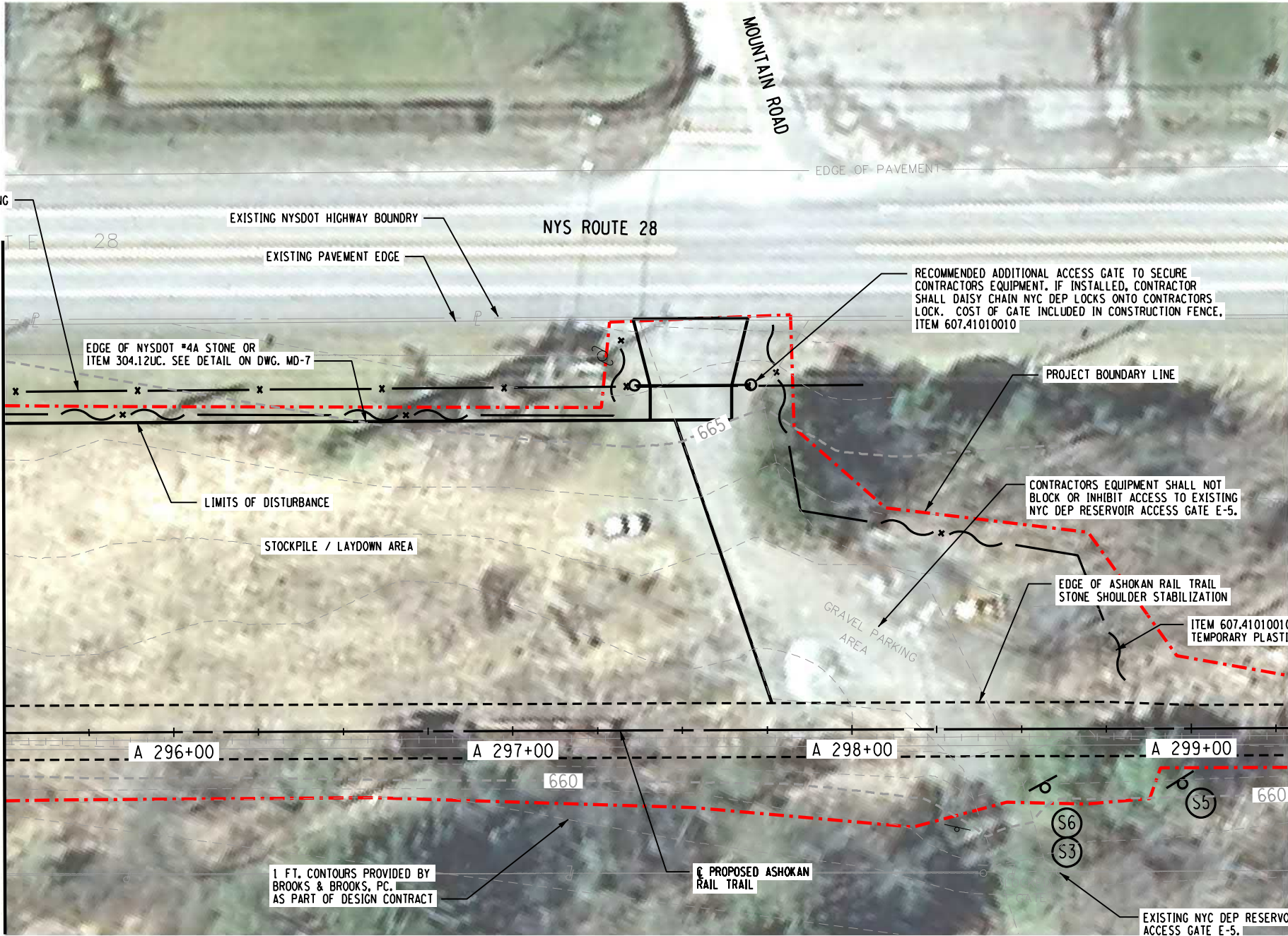
SHOKAN STATION ACCESS ROAD AND LAYDOWN AREA PLAN MATERIAL STORAGE, LAYDOWN, OR STOCKPILING IN SHADED AREAS ONLY. STONE AND GEOTEXTILE FABRIC SHALL BE REMOVED IN THESE AREAS POST CONSTRUCTION OF TRAIL TO EXPOSE UNDERLYING SOILS BELOW GEOTEXTILE FABRIC. REMOVAL OF STONE TO BE PAID FOR UNDER ITEM 203.02.
