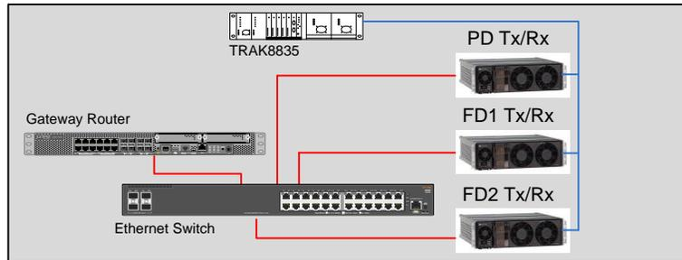
**Figure 1-2: Basic Diagram of Ulster Analog Simulcast Remote Site with FD & PD Channels**
