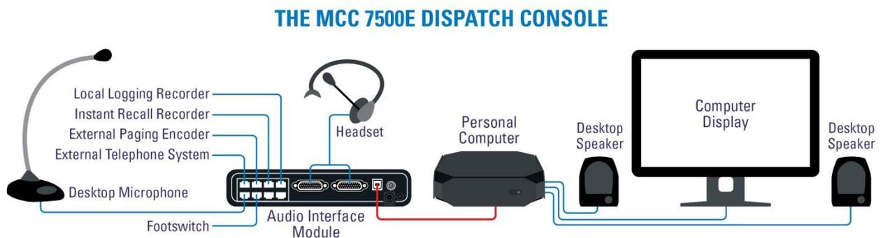
**Figure 1-2: Motorola MCC 7500E Dispatch Console Hardware Architecture Diagram is for illustration purposes only – see section 1.2 for list of components**
